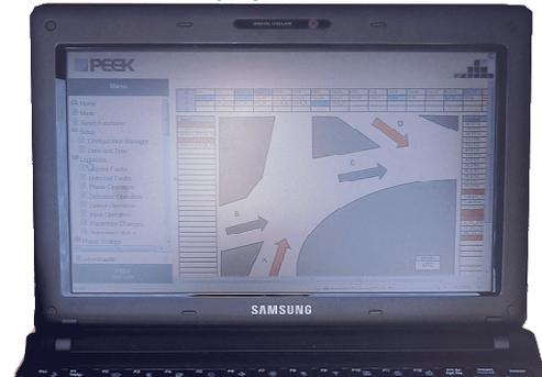
In addition to the traffic signal controller, the Outstation Monitoring Unit (separate from the MOVA unit for compatibility with the Remote Monitoring System (RMS)), the MOVA unit and the low-cost CCTV system are also equipped with Ethernet connections, which allows remote communications to be carried out via a broadband telephone connection, by assigning each sub-system with a unique IP address.
